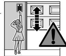
Caution notices warning about the trap risk must be permanently fixed in a conspicuous place or in the proximity of the permanently installed buttons used to actuate the operator. The construction of the garage ceiling must be such that safe, secure anchoring of the operator is guaranteed.
