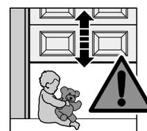
Make sure that neither persons nor objects are located within the door's range of travel. Initial function checks as well as programming or extending the remote control should always be carried out from inside the garage.
